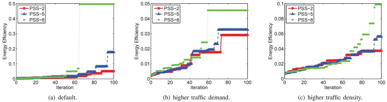
Fig. 3. Energy efficiency comparison under different network parameters with 5 channels.
