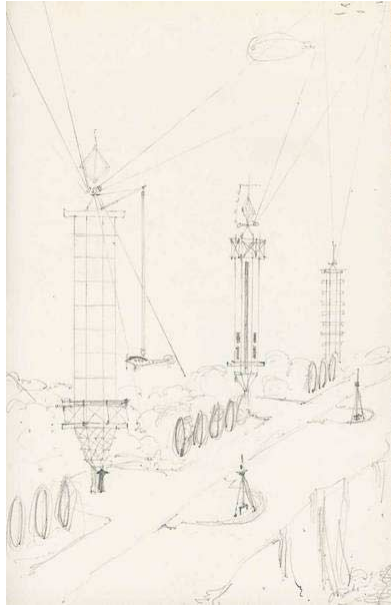
R.B. Fuller elevation, plan & perspective - Towers with wind generators aloft - Chicago, 1928
