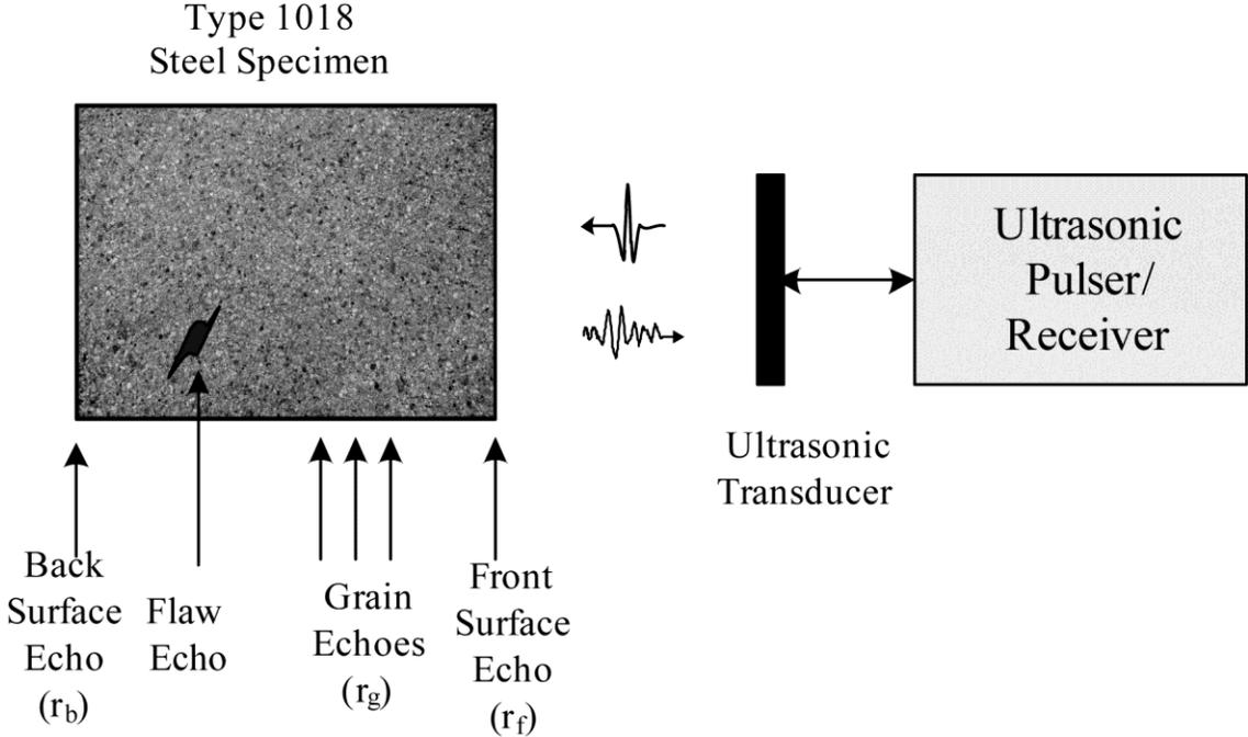
Fig. 1.1. Ultrasonic testing setup using a steel block (type 1018, grain size 50 $\mu$ m) to evaluate the characteristics of flaw echo and grain scattering.
