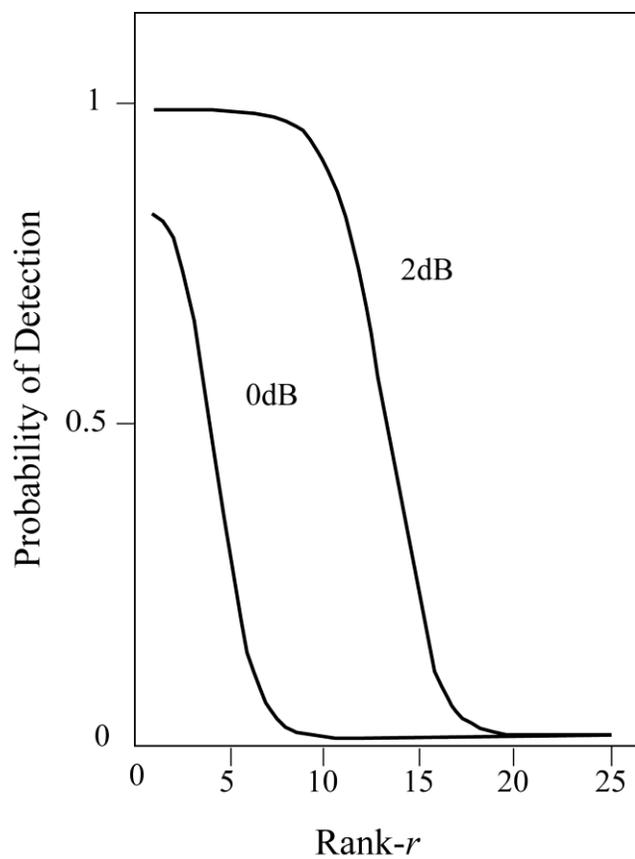
Fig. 1.8. Probability of detection of Chi distributed target-plus-clutter in Weibull distributed clutter for various ranks of OS filters with  $n=25$  and the probability of false alarm set at 0.001
