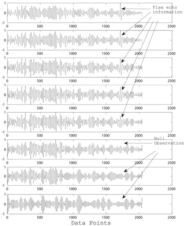
Fig. 1.5. Observation channels (output of split-spectrum processing) where the null observations are in higher frequency bands.
