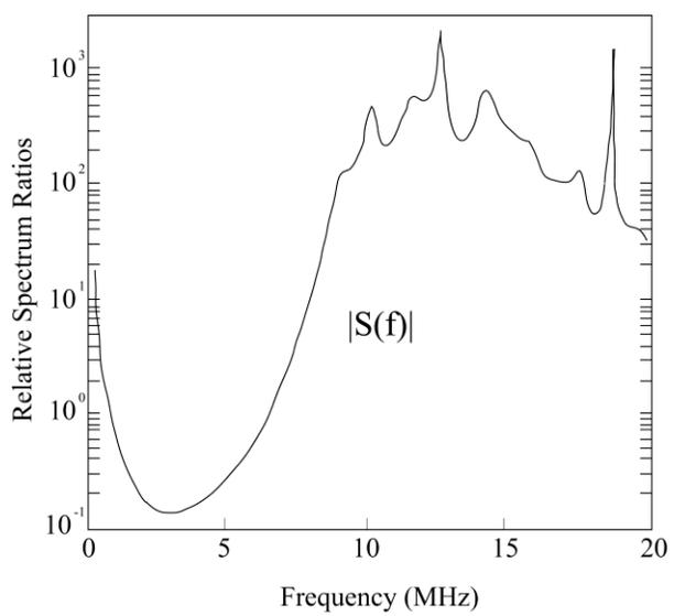
Fig. 1.6. a) Attenuation transfer function, b) Scattering transfer function
