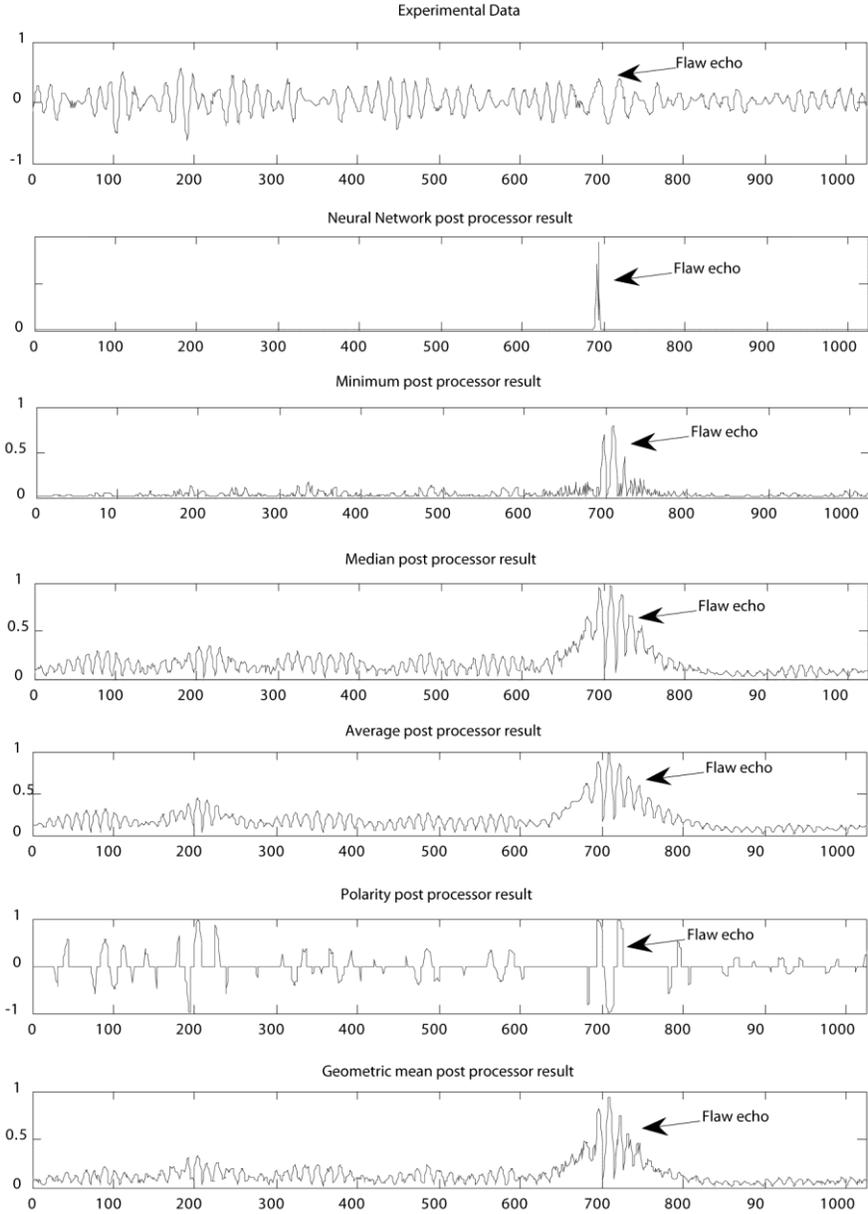
Fig. 1.16. Comparison of detection results when SSP channels covering the low frequency region
