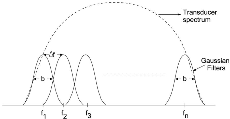
Fig. 1.4. Frequency bands in split-spectrum processing, where  $b$  is the filter bandwidth,  $\Delta f$  is the frequency step within the bands, and  $f_1 \dots f_n$  are the subbands' center frequency.
