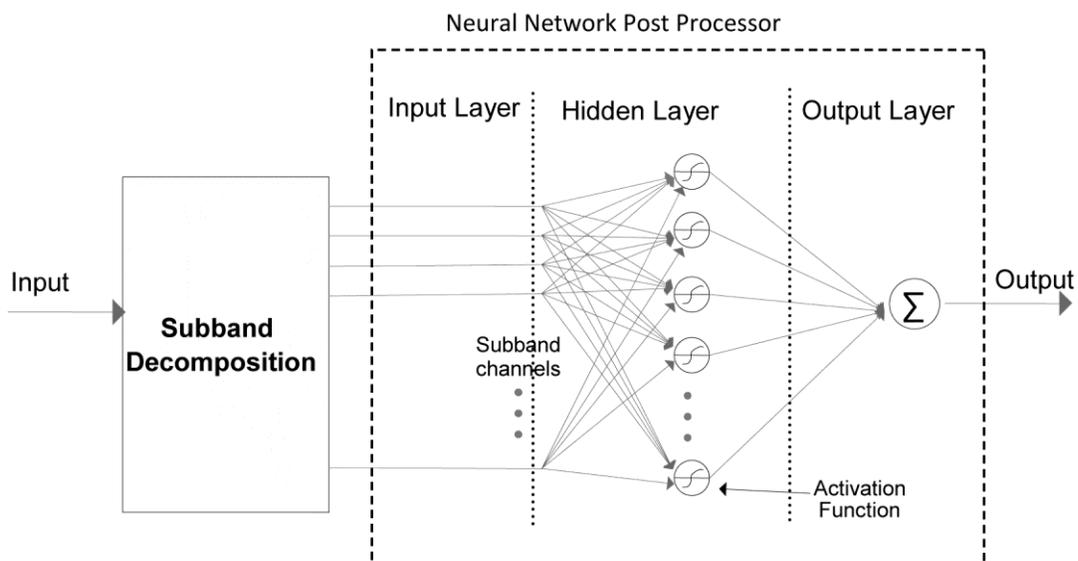
Fig. 1.11. Three layer feed-forward neural network for SSP flow detection
