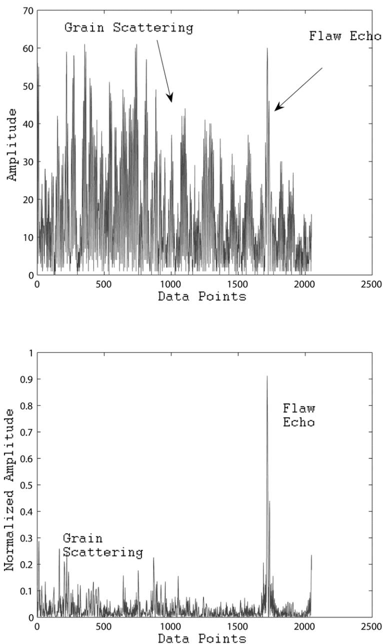
Fig. 1.2 Ultrasonic experimental flaw signal (top trace) and frequency-diverse minimum detector result (bottom trace). A broadband ultrasonic transducer with 5MHz center frequency and a pulser/receiver (Panametric, type 5052) operating in pulse-echo mode is used for the experimental measurement.
