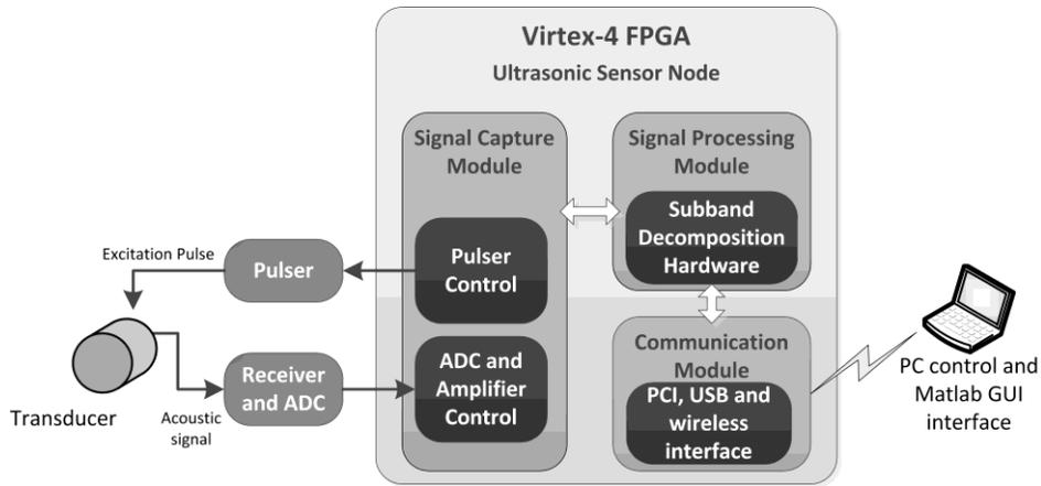
Fig. 1.18. FPGA based real-time ultrasonic flow detection system
