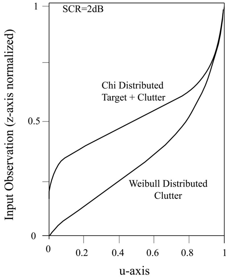
Fig. 1.7. Inverse distribution functions of Chi-distributed target-plus-clutter and Weibull-distributed clutter
