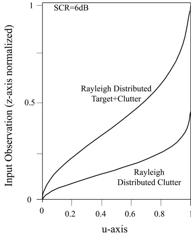
Fig. 1.9. Inverse distribution functions of Rayleigh-distributed target-plus-clutter and Rayleigh distributed clutter
