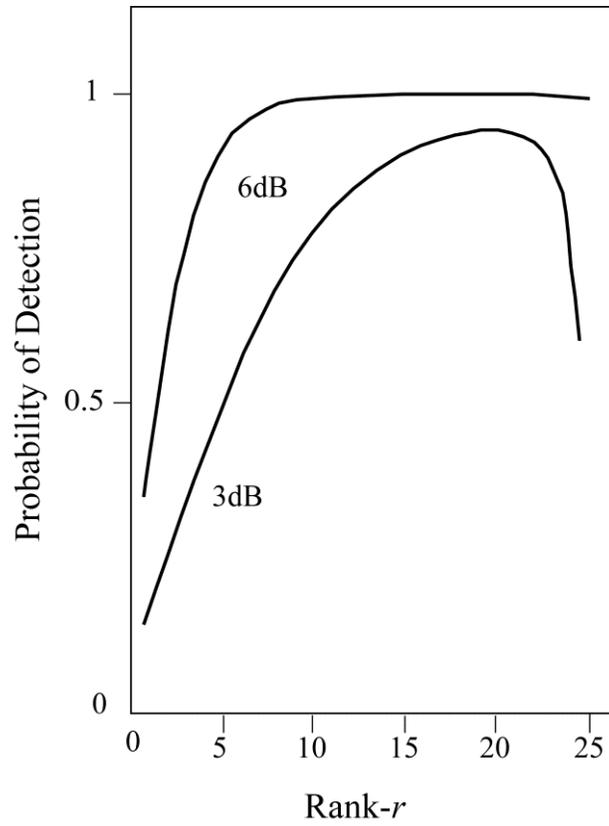
Fig. 1.10. Probability of detection of Rayleigh distributed target in Rayleigh distributed clutter for various ranks of OS filters with  $n = 25$  and the probability of false alarm set at 0.001.
