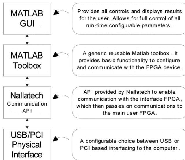
Fig. 1.19. Software interface designed for ultrasonic flow detection system
