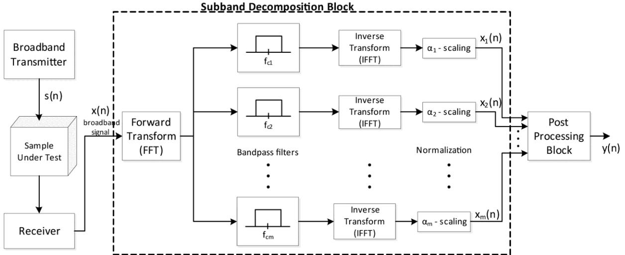
Fig. 1.3. Frequency-diverse ultrasonic flaw detection system based on split-spectrum processing
