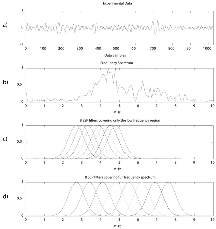
Fig. 1.15. Experimental data in time domain, frequency domain and frequency bands of SSP filters
