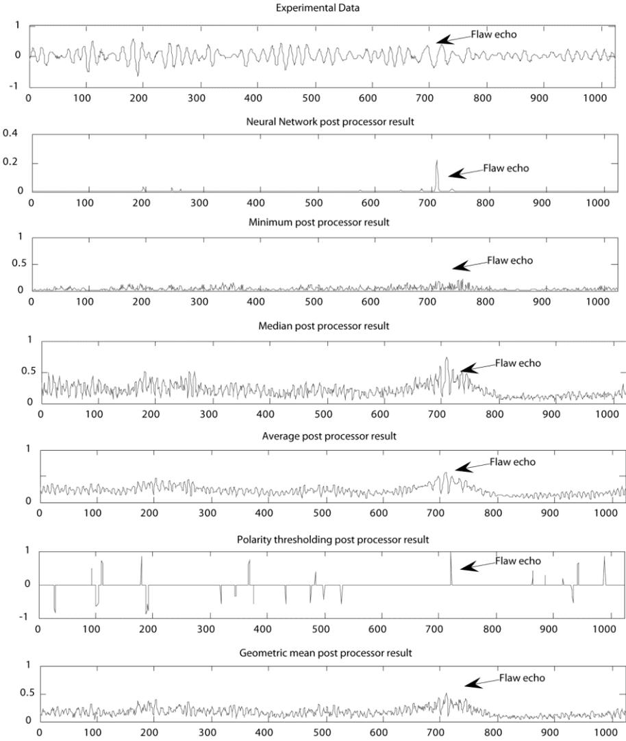
Fig. 1.17. Comparison of detection results when SSP channels covering the full frequency range
