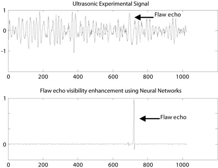
Fig. 1.14. Detection results using Neural Network based SSP
