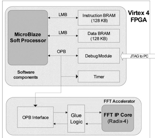
Fig. 1.20. Hardware/Software co-design components
