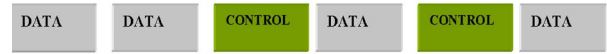
Fig. 6. The control packets are included randomly between data packets to avoid complete drop of control packets by the malicious node.
