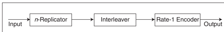
Fig. 2. A schematic representation of a rate 1/n turbo encoder. The box labeled n -replicator represents a device which successively delivers n times its input symbol. The interleaver changes the order of the symbols in its input sequence, and the rate-1 encoder outputs symbols which combine a number of its successive input symbols. The n -replicator is the sole of the devices in the scheme to generate the necessary redundancy.
